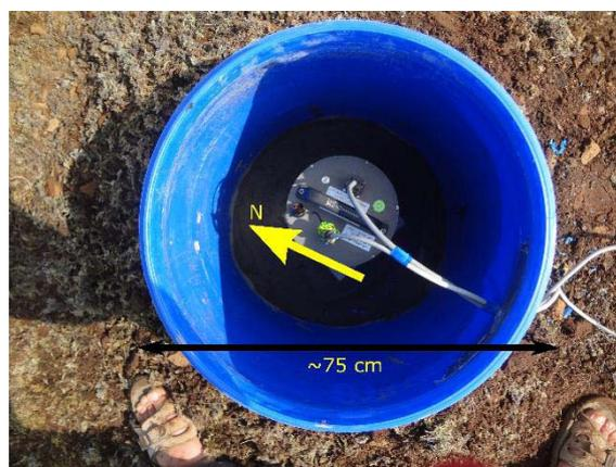
A 16 Gbyte seismometer typically filled the memory in 10.5 months, so we serviced the array twice: once in early July, which is the earliest we could access the area; and again in early September. This also gave us the opportunity to replace any failing components at the sites (we found the GPS antennae to be often the most likely component to fail during deployments).
