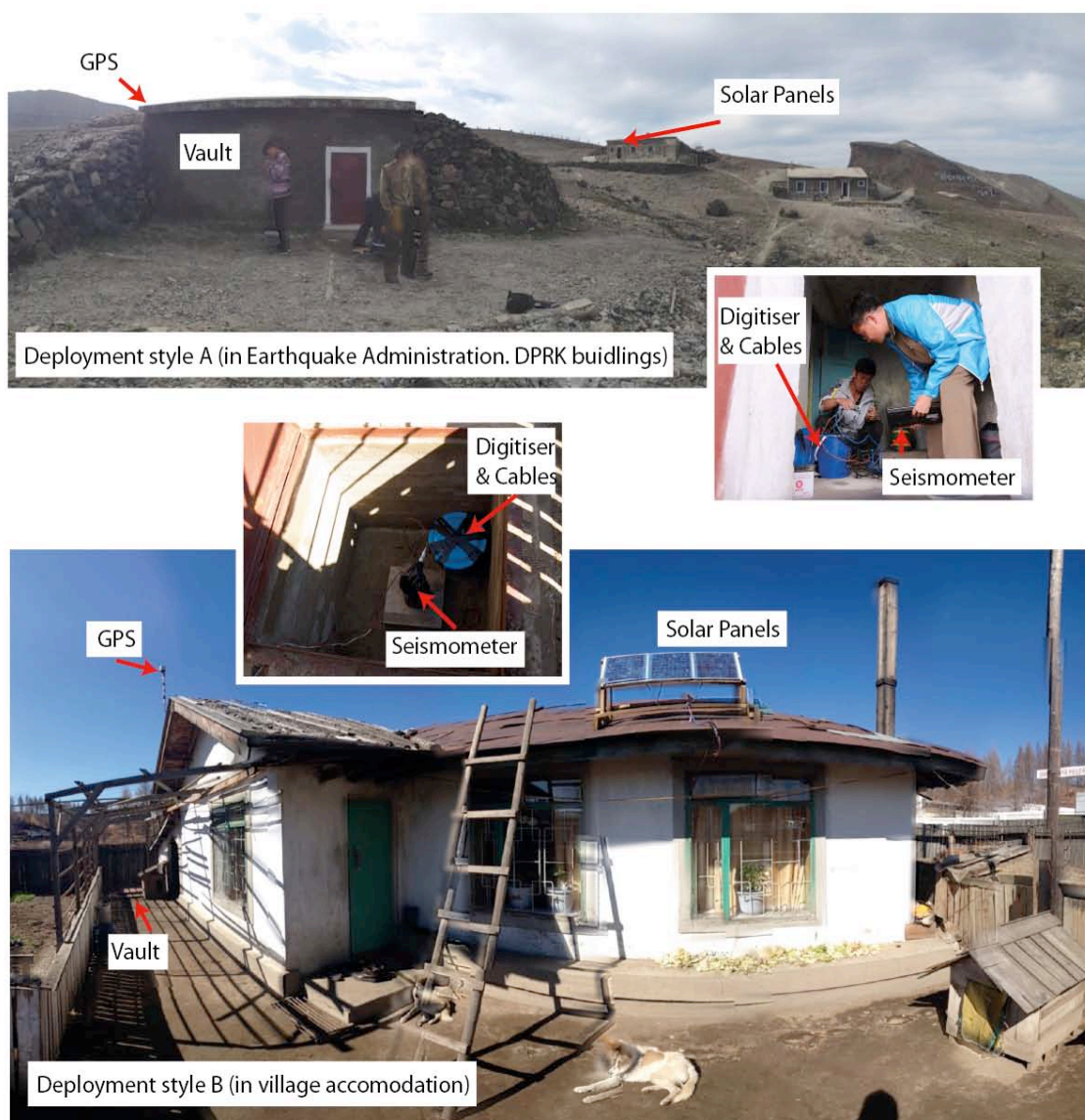
Figure 2. Deployment styles for A) deployment within Earthquake Administration, DPRK sites (top) and B) deployment within village accomodation (bottom). All stations were deployed in purpose built vaults.
