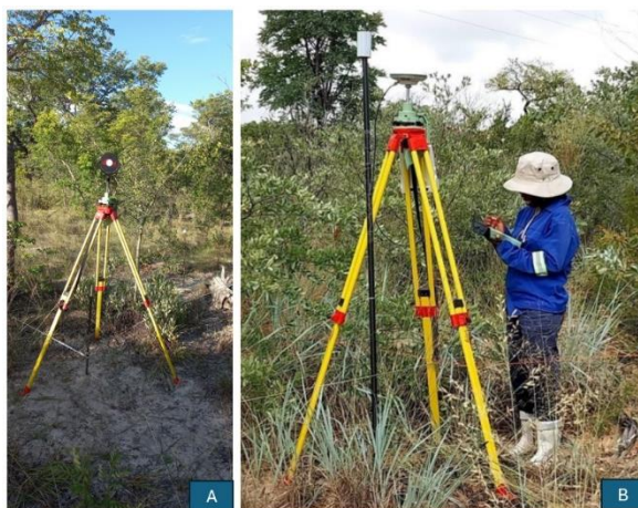
Figure 3: Reflectors used as tie points during the scanning. A - a flat reflector of 5 cm used in the corner of the plot. B – A white reflector of 10 cm length erected on a black pole. If the overstorey in the plot is dense, reflectors are put on high poles to ensure that it is seen over the bushes.
