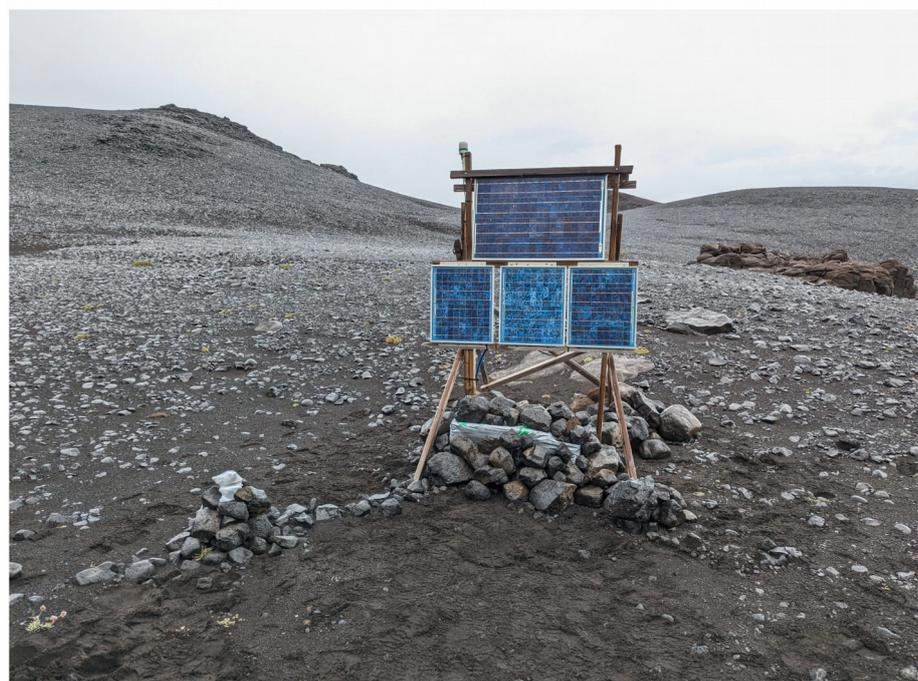
**Figure 2:** Two examples of standard station deployments in the Highlands. In both photos, the panel stand, plastic box housing the regulator and batteries, breakout box (wrapped in plastic), and GPS antenna, are clearly visible. Where available, volcanic rocks are used as ballast and protection.
