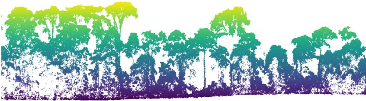
Figure 2 – A 250 m wide cross section of the LiDAR data covering one of our field plots in Gabon with the tallest tree reaches over 50 m. The data was collected over two separate flights.
