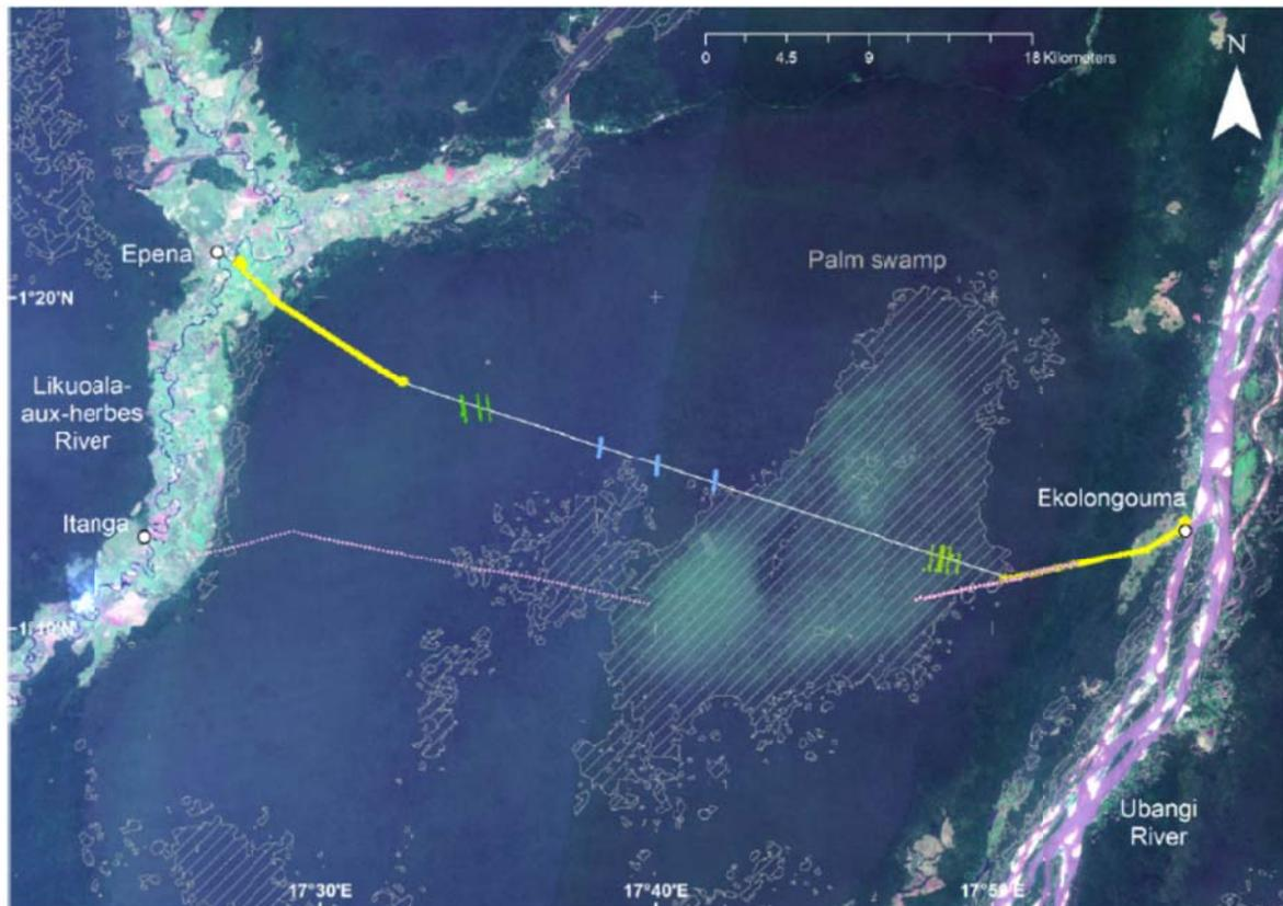
**Figure 6** - The locations of acquired data UAV LiDAR (yellow), IceSat (green), IceSat2 (blue) and the area believed to be palm swamp (white hatched). A white line joins the LiDAR transects forming a path between the peat edges 43.8 km long, compared to 43.3 km direct-line distance. Background image is a Sentinel-2 composite, Copyright European Space Agency. The base station area shown by white dots. Image taken from our own published paper by Davenport et al. [7]
