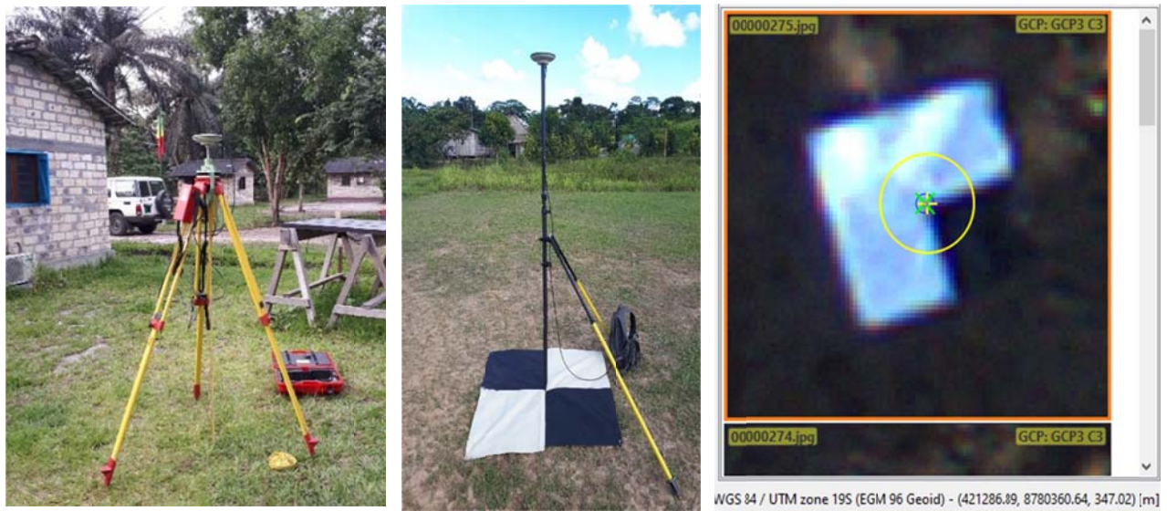
Figure 3 – Base station set up in the village of Epena, Republic of Congo (Left), the data from which was used to correct the UAV flight trajectory, and the data collected from the rover receiver, which was used to collect GCPs (centre). These GCPs were clearly visible in the DAP (right image) and the LiDAR data. The estimated position is identified with a blue dot. The distance to the centre of the target (defined manually) was 0.01, 0.01, 0.01 (x,y,z).
