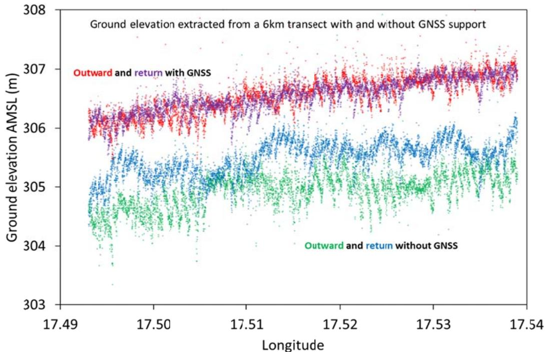
**Figure 4** – Ground elevation as estimated from the LiDAR data collected from our DT26 UAV equipped with a Trimble GNSS receiver pre- (green and blue) and post-correction (red and purple). The data comes from one 12 km transect.
