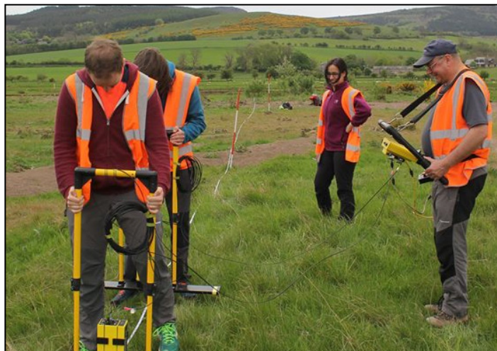
Figure 2. The use of the 100 MHz antenna to collect a profile at Thropton grid.
