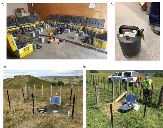
Figure 3: a) CMG-6TD huddle test in the Gisborne field centre. b) CMG-6TD instrument. c) Example CMG-6TD site with battery box to the left of solar panel and tarpaulin below solar panel to prevent grass growth. d) example site location where battery box has been positioned beneath solar panel. During servicing it was discovered that some solar panels had fallen forward and the presence of these boxes helped maintain them at a useful angle.
