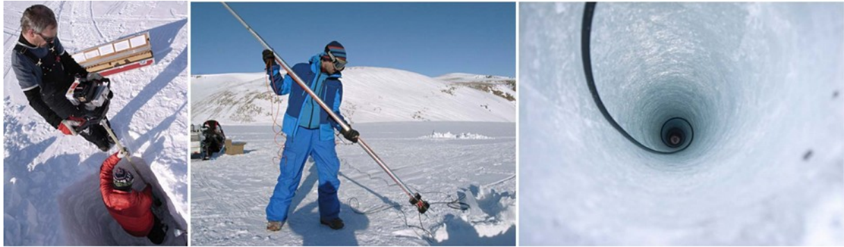
Figure 5: Drilling and deployment of a borehole. Photos: GlacioBurst field team
