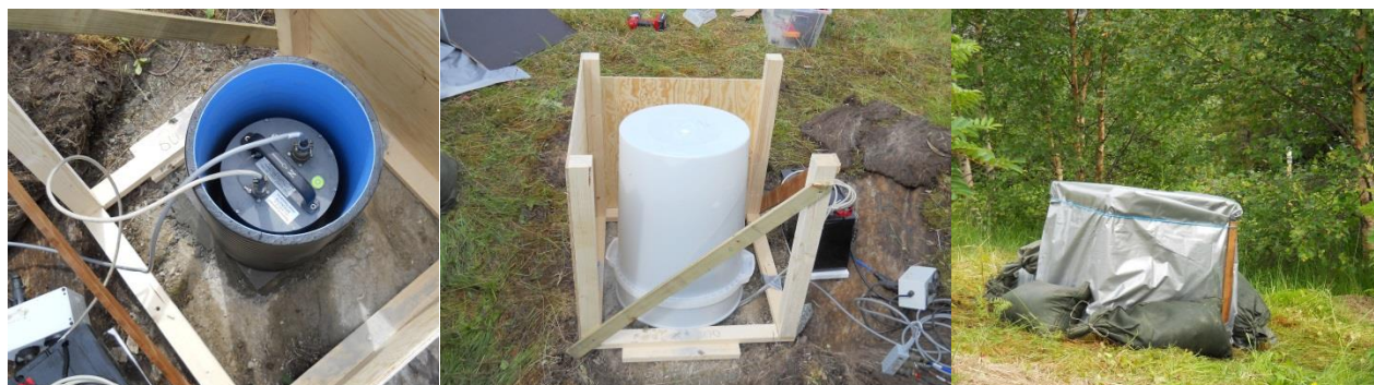
Fig. 4. Stages in construction of one of the outdoor sites. See text for details. Power was supplied by cable from a house nearby. The battery box is largely hidden behind the instrument box in the right hand photograph.
