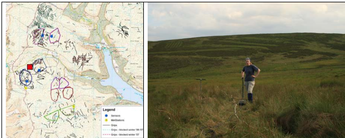
Figure 1: Map of the RSPB Lake Vyrnwy Reserve site and experimental set up (left). Coloured polygons are the control (solid line) and treated (dashed line) grip-blocked areas for each catchment. Red square shows the location of the pilot GPR study. Right panel shows site and survey operation (image N. MacBean).
