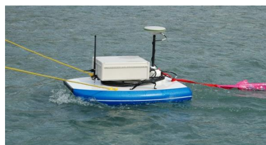
Figure 5. Sontek S5 acoustic Doppler current profiler, with integrated Leica GX1230 GPS receiver
