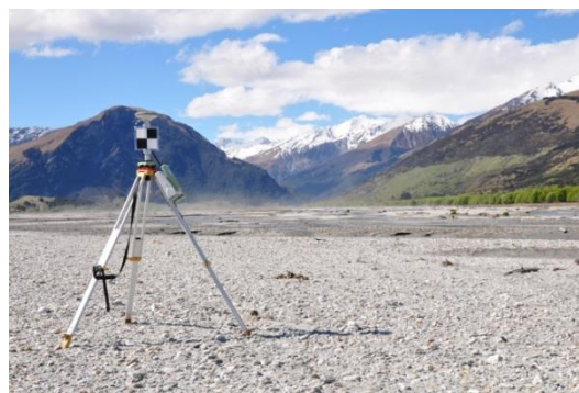
Figure 4. GPS located survey targets used for registration.
