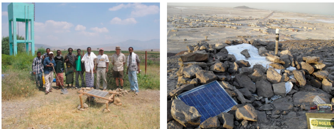
Figure 3. left panel shows a typical subsurface deployment and the right panel shows a typical subaerial deployments with both the sensor and battery/breakout box housing covered with a cairn of rocks and reflective foil.
