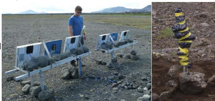
Bench design solar panel stand with mounted GPS
