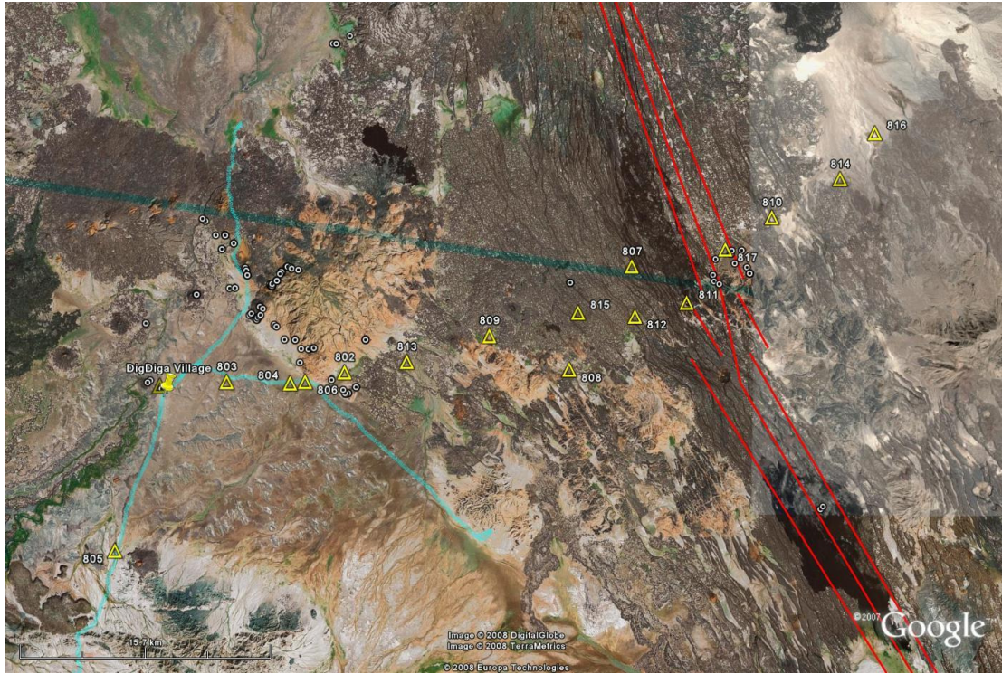
Figure 2. MT sites (yellow triangles) along a profile approximately perpendicular to the axis of dyking (red lines). Small circles are petrological sampling sites. DigDiga village was our field base.
