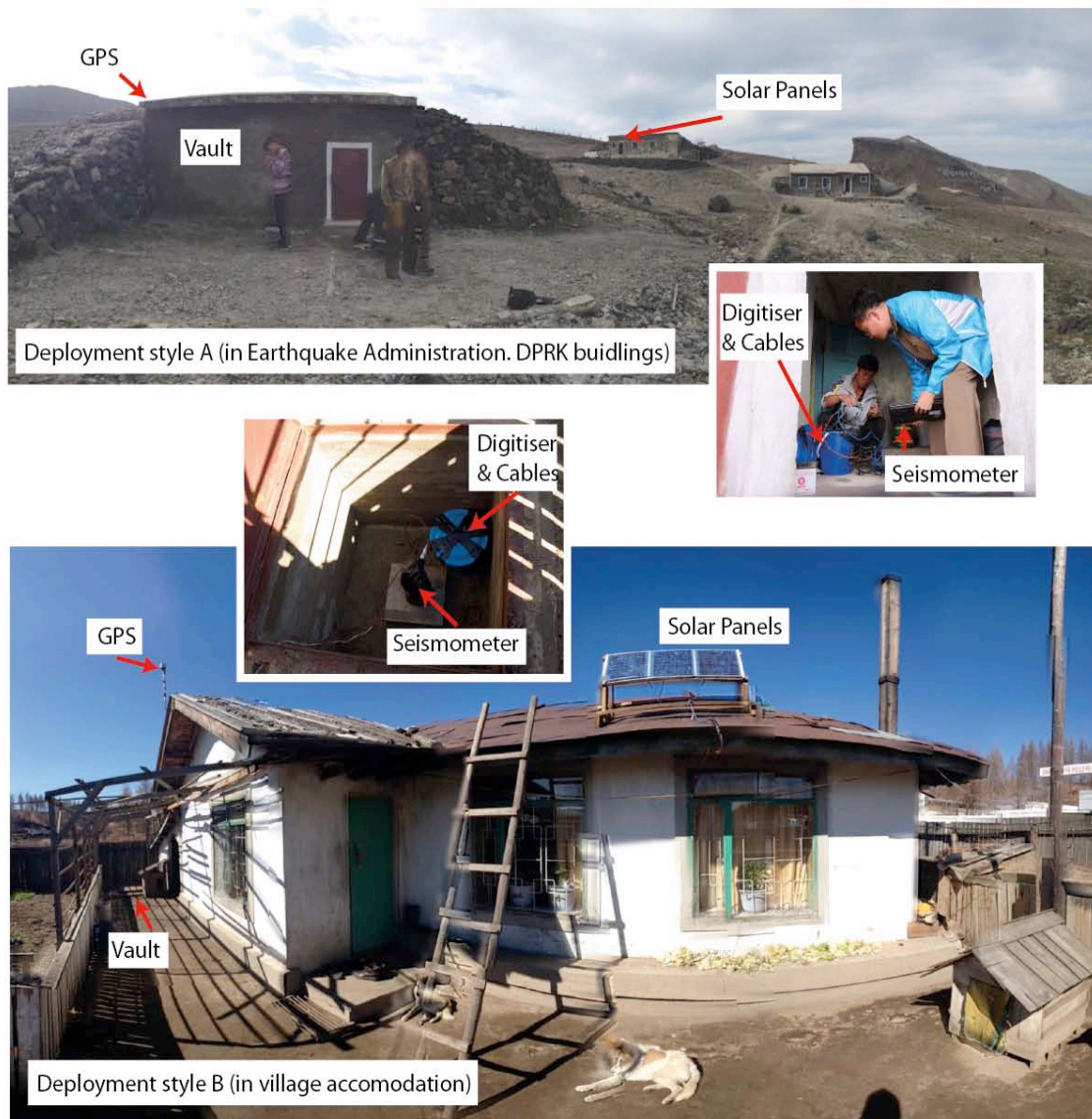
Figure 2. Deployment styles for A) deployment within Earthquake Administration, DPRK sites (top) and B) deployment within village accomodation (bottom). All stations were deployed in purpose built vaults.
