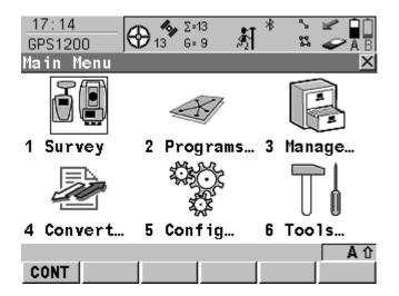
To move around the menu system use the arrow keys on the keypad followed by the ENTER key or F1 (CONT)
