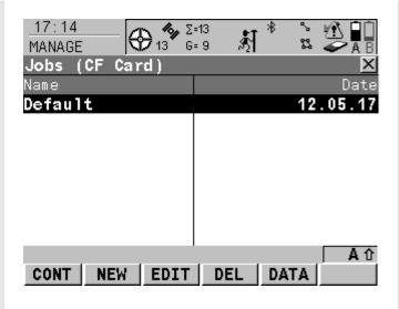
Before starting a new survey, it is recommended to delete any previous jobs from the memory card to ensure the maximum amount of free space (at a recording rate of 2Hz, you should have room for at least 48 hours of data on the supplied card).
