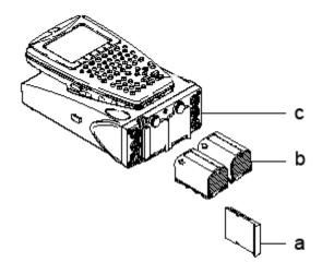
Unscrew the left hand battery holder on the receiver (c) and insert the Compact Flash card (a). CAUTION: The arrow must face into the unit and the label with the arrow on it must face towards the right
